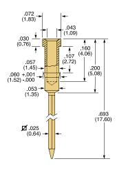
Materials: Brass, gold plated Mounting Hole Size: .085 (2.15) Applications: Designed for use in original GenRad interface boards.
