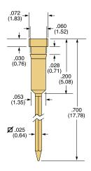
SIP-90-3 Materials: Brass, gold plated Mounting Hole Size: .055 (1.40) Applications: Designed for use in original Zehntel interface panels.
