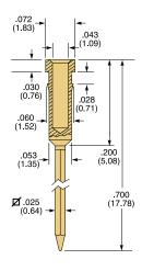
SIP-90-4 Materials: Brass, gold plated Mounting Hole Size: .055 (1.40) Applications: Designed for use in original Factron interface panels. SIP-90-4 replaces SIP-90-1.
