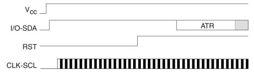
After a successful ATR, the Protocol and Parameter Selection (PPS) protocol, as defined by ISO 7816-3, may be used to negotiate the communications speed with CryptoMemory devices 32 Kbits and larger. CryptoMemory supports D values of 1, 2, 4, 8, 12, and 16 for an F value of 372. Also supported are D values of 8 and 16 for F = 512. This allows selection of 8 communications speeds ranging from 9600 baud to 153,600 baud.
