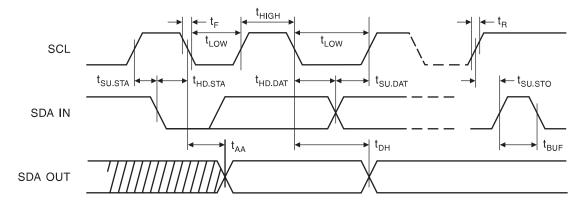
Figure 3. Write Cycle Timing:
